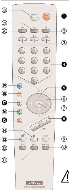
The remote control sends commands to the TV set by means of an infrared signal. You must point it towards the TV set when using it. Note that the remote control may interfere with the operation of other devices which use infrared signals (such as infrared headphones).
